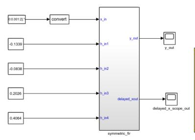
This example shows how to use HDL Coder to check, generate, and verify HDL for a fixed-point symmetric FIR filter. In MATLAB, type the following: checkhdl('sfir\_fixed/symmetric\_fir') makehdl('sfir\_fixed/symmetric\_fir') makehdl(b('sfir\_fixed/symmetric\_fir') Or double-click the blue button at the bottom to see the dialog.
