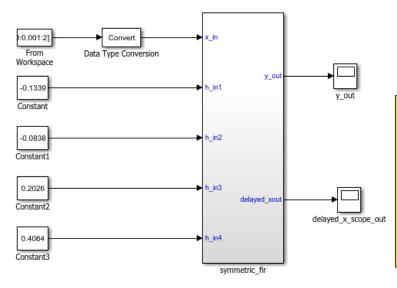
This example shows how to use HDL Coder to check, generate, and verify HDL for a fixed-point symmetric FIR filter. In MATLAB, type the following: checkhdl('sfir\_fixed/symmetric\_fir') makehdl('sfir\_fixed/symmetric\_fir') makehdltb('sfir\_fixed/symmetric\_fir') Or double-click the blue button at the bottom to see the dialog.
