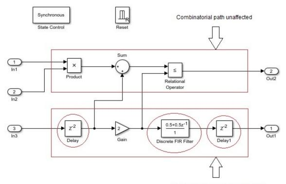
Sequential blocks get reset based on Synchronous Subsystem reset control
