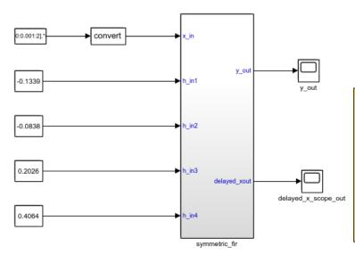
This example shows how to use HDL Coder to check, generate, and verify HDL for a fixed-point symmetric FIR filter. In MATLAB, type the following: checkhdl('sfir\_fixed/symmetric\_fir') makehdltb('sfir\_fixed/symmetric\_fir') makehdltb('sfir\_fixed/symmetric\_fir') Or double-click the blue button at the bottom to see the dialog.
